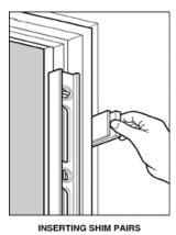
Drive a 8d finishing nail through the jamb, shims and partway into the stud at each hinge point. Do not drive the nails home yet. Check for plumb and adjust as necessary.
