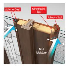
G Lip-lite frame (shown right) features a compression seal against weather on the outside of the door and an adhesive seal against weather on the outside of the glass. Flush-glazed glass (shown left) is built directly into the door without a Lip-lite frame, featuring a high-performance adhesive weather seal inside and out.
