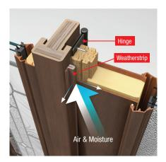
4 Hinges position the door to properly compress the weatherstrip to help form a tight, even seal against air and moisture infiltration when the door closes.
