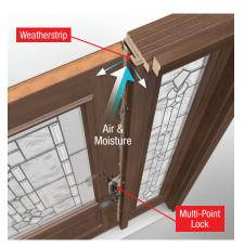
6 Multi-point locking system (recommended) engages the door and frame at three points from top to bottom for enhanced security while helping to preserve the weatherstrip's seal even under wind pressure.
