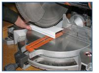
3. Cut jamb cover & brickmould.
