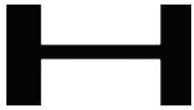
Supplemental Aluminum Stiffener for Savannah, Newport, and Bellhaven for Rail Lengths over 8'
